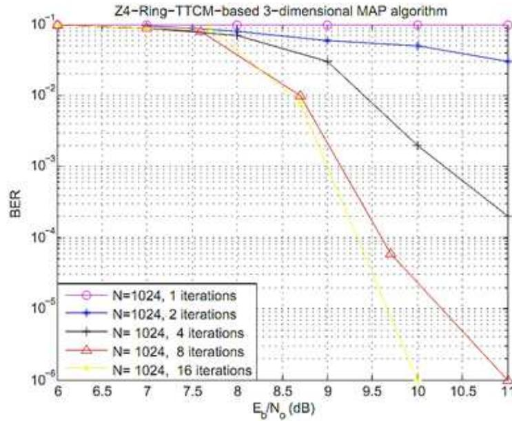
**Figure 8: The Performance of the  $\mathbb{Z}_4$ -Ring-TTCM System-Based 3-Dimensional MAP Algorithm**
