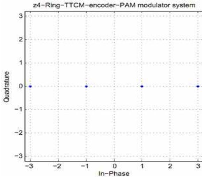
**Figure 6: The Scatter Plot of Constellation Points for the  $\mathbb{Z}_4$ -Ring-TTCM Encoder-Modulator-Based PAM Modulator**
