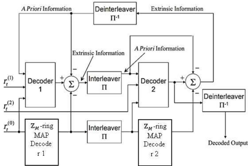
Figure 4: The  $\mathbb{Z}_M$ -Ring-Turbo Decoder
