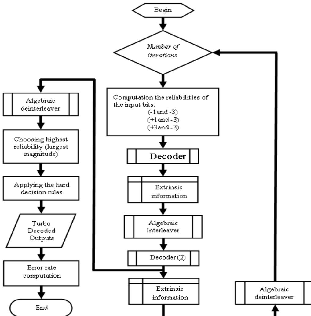
Figure 5: Flow Chart of the  $\mathbb{Z}_4$ -Ring-TTCM Decoder Algorithm
