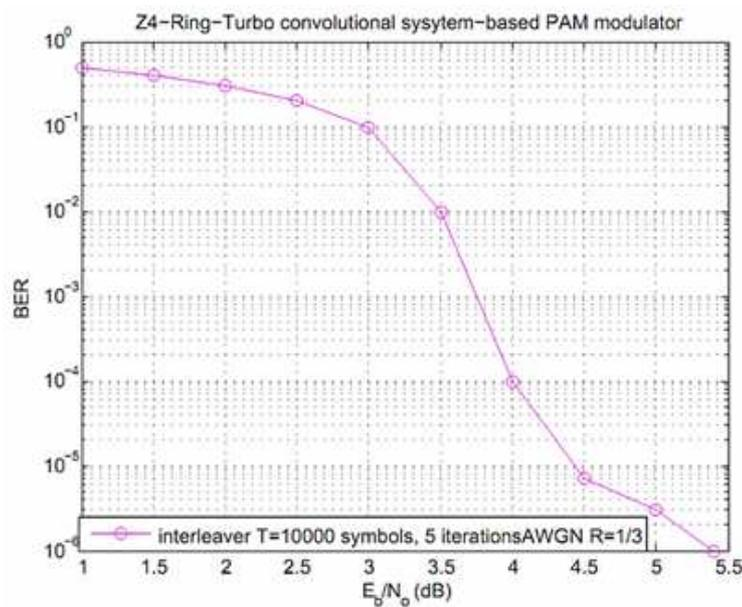
**Figure 7: The Performance of the  $\mathbb{Z}_4$ -Ring-TC System-Based PAM Modulator**
